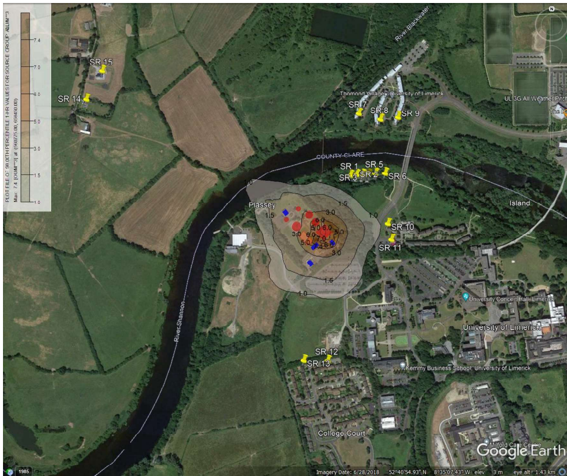
Figure 7-4: Proposed Development to Castletroy WwTP - Predicted Worst-Case 98th Percentile of Hourly Average Odour Concentrations 2021.
